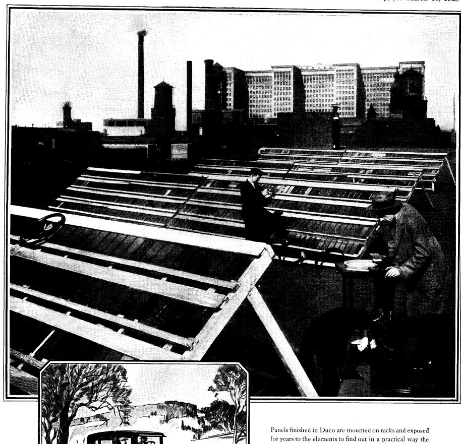
Panels finished in Duco are mounted on racks and exposed for years to the elements to find out in a practical way the durability of Duco under the action of sun, wind, and rain, hail and snow, the dirt from city streets, and the soot from nearby chimneys.
