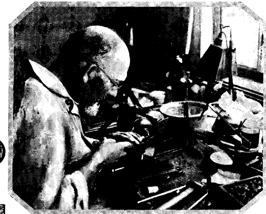
An Amsterdam diamond cutter at work. The stone is imbedded in cement and is cut by another diamond
