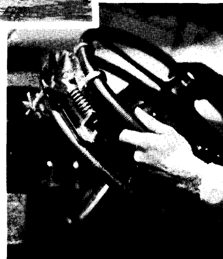
Below. Steering ease is another big factor in safety and driving comfort. Shown here is a "duplicate" steering wheel which the engineers have developed to measure steering effort.
