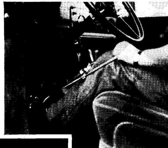
Above. This special instrument, developed by the Proving Ground engineers, measures clutch pedal pressure. Still other devices have been developed to record acceleration and deceleration to a degree of accuracy previously unknown.
