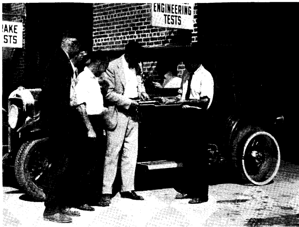
Above. The large picture shows a group of Proving Ground engineers examining the precision device described at the upper right. The "fifth wheel," shown at the rear wheel of the car, is another specially developed instrument which measures exact speed.
