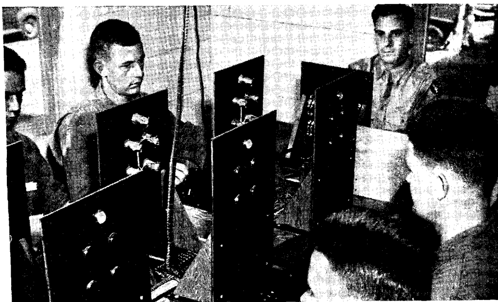
When lights on board flash, cadets must throw a corresponding switch on the table, thus enabling Staff Sergeant Klapper (in background) to test their reaction time
