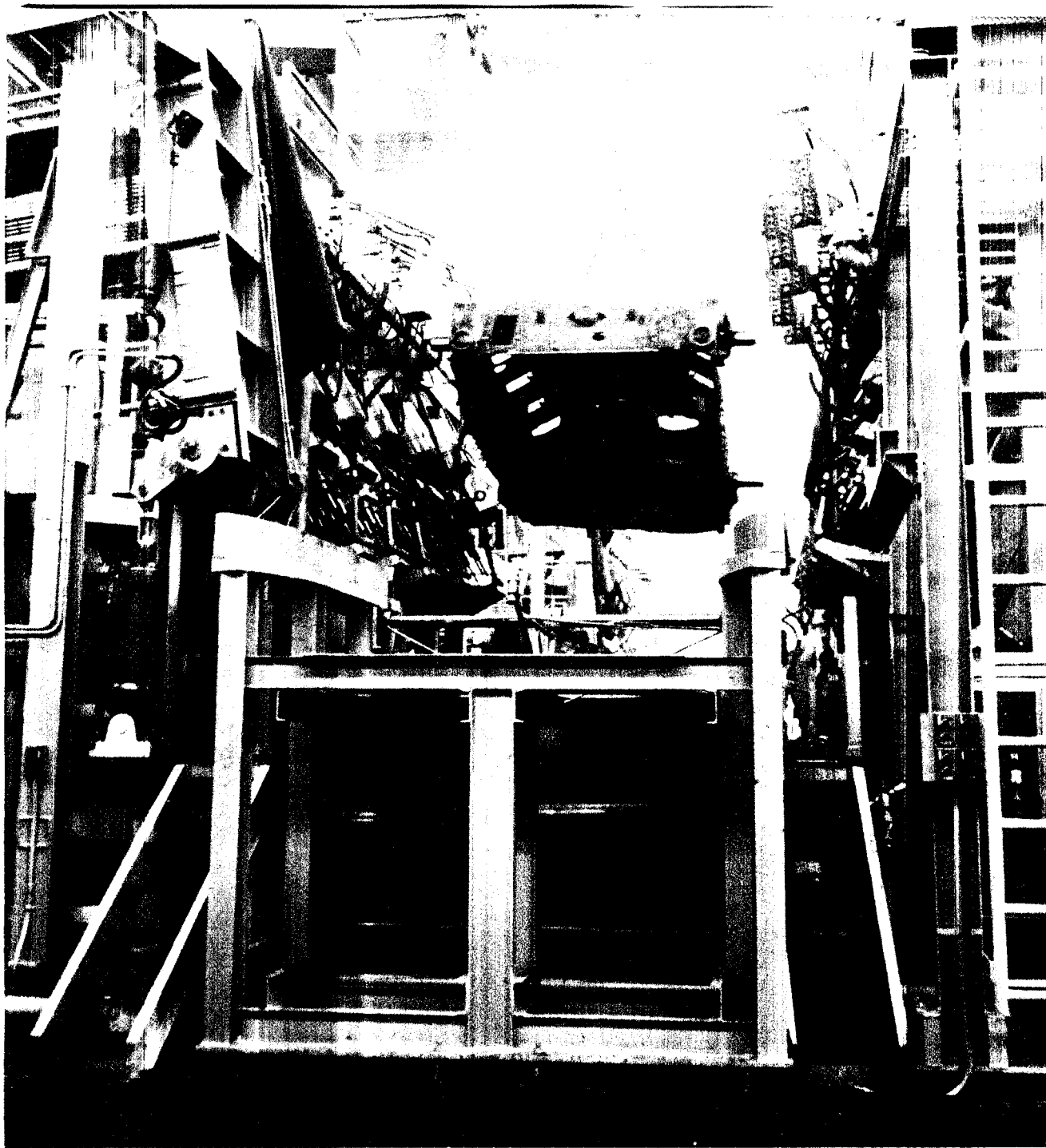
Crane lowers tank hull into "Queen Elizabeth" machine, which drills 100 holes simultaneously
