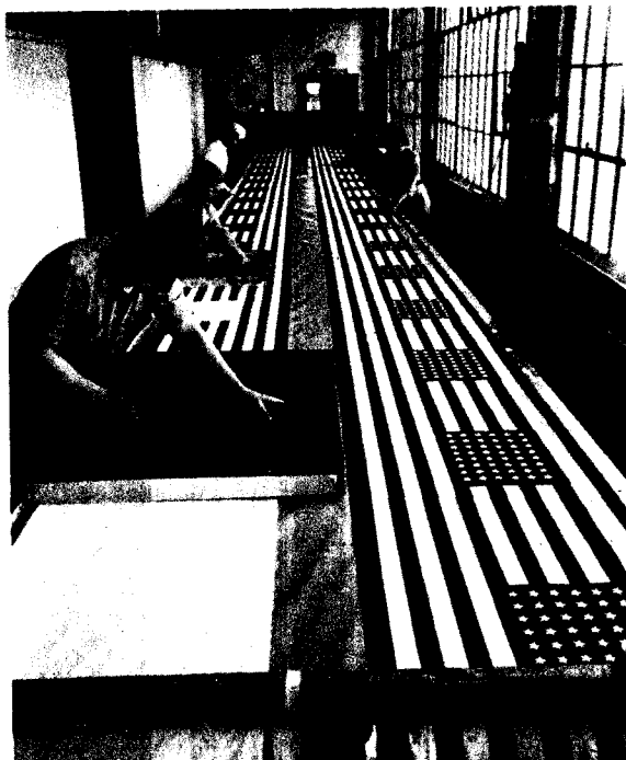
Annin's small flags are silk-screen printed by pressing colors through patterns on silk
