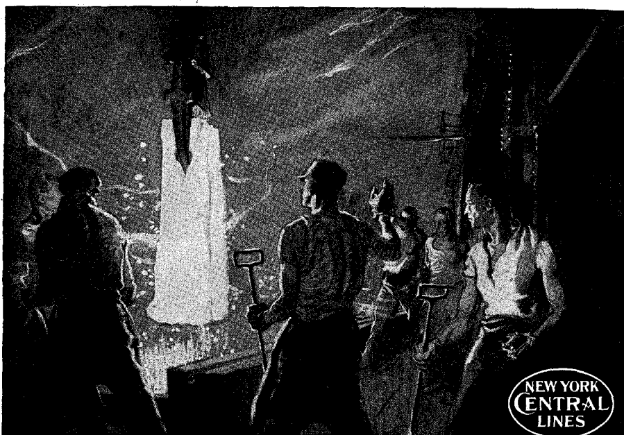
Steel ingot being taken from reheating furnace preparatory to rolling into rails
