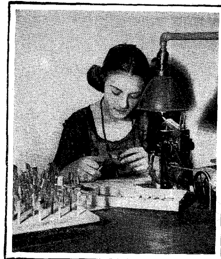
MOUNTING THE PLATE ON THE SUPPORTING LEADS OVER THE GRID AND FILAMENT
