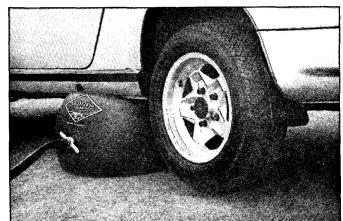
is made of PVC-coated nylon mesh with welded seams (the same construction used for giant transport bags that hold 75 tons of cement). Large 21" diameter means car can not roll off jack. Needs only 1" clearance to fit under vehicle. Great for getting out of ruts or jacking on ice, snow, uneven ground. Compact enough to store in
