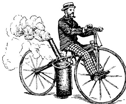
Steam velocipede of 1868 proved useless since firebox was too close to ground.
