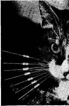
Glass keeps cat's whiskers dry. Corning has developed a new way to mass-produce short lengths of small glass tubing accurate to a few thousandths of an inch. This material was found to be perfect for encasing new miniature diodes. These tiny devices—a lot like the cat's whiskers and crystals of old radio sets—are used to replace vacuum tubes in certain jobs. And once hermetically sealed in their glass cases, they're tough, compact, and they almost never wear out.
