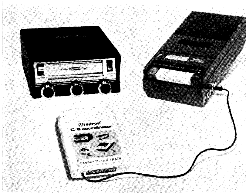
This adapter channels the output of a cassette recorder (or radio) through an automobile's 8-track cartridge player.
